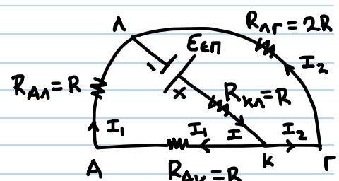
$$R_{OJ} = R_{12} + R_{KA} = 2R \quad \text{οπότε} \quad I = \frac{\mathcal{E}_{\text{en}}}{R_{OJ}} = \frac{B \pi l^2}{R \cdot T}$$
