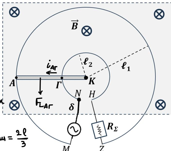
$$R_{AG} = P \frac{l_{AG}}{S} = \frac{2}{3} P \frac{l}{S} = \frac{2}{3} R_{AG} = \frac{2}{3} 3 \Omega$$
