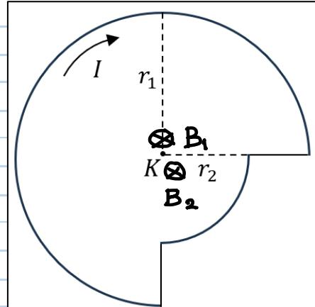
$$B = \frac{\mu_0}{4\pi} \frac{I}{r} \varphi \quad \text{αφού } \vec{r} \perp d\vec{l} \quad \text{και } \eta\vartheta = 1$$
