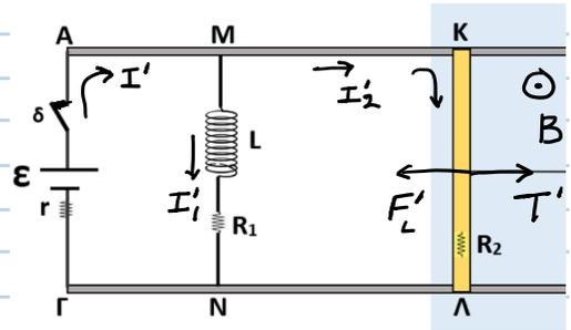
$$V_{R_1} = V_{R_2} \Rightarrow I'_1 R_1 = I'_2 R_2 \Rightarrow I'_1 = 3I'_2, \quad I' = I'_1 + I'_2 = 4I'_2 \Rightarrow I'_2 = \frac{I'}{4} = 1 \text{ A}$$
